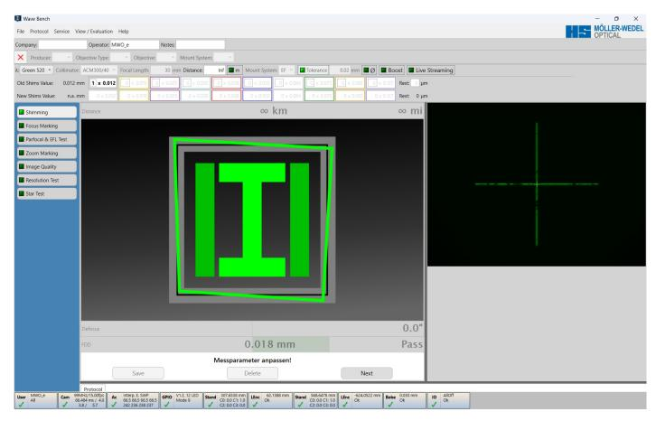
In addition to precise shimming at any distance, the software can calculate the best new shim combination for the lens being tested. When shimming, the square deviation gives a first impression of the image quality. If the square does not look good enough, the image quality can be assessed in detail in terms of astigmatism, coma and overall image quality.
