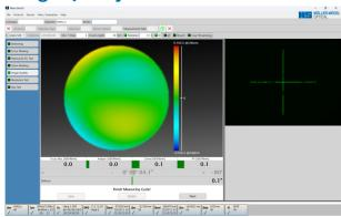
In addition to checking the focus marking or generating user marks for the follow focus, the bench can also check the parfocal tuning. Parfocal shimming can be performed as an option. With image quality, astigmatism, coma and overall image performance can be evaluated and recorded as comparable figures.
