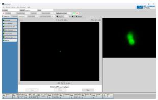
The optional tests can be used for detailed evaluation. Will the lens achieve the expected contrast at HD, 4K or 8K? The MTF evaluation provides contrast values for the selected resolution.
